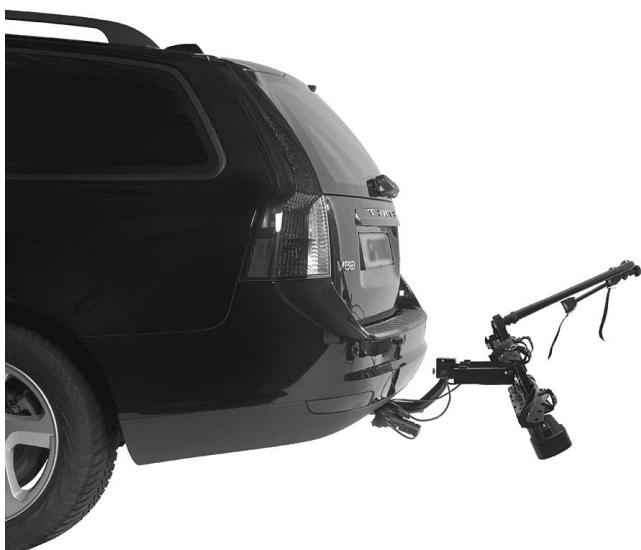
By pushing the entire carrier up, the tilting mechanism is locked again (you hear a click). Make sure to always secure the handle again by sliding this to the locking position.
