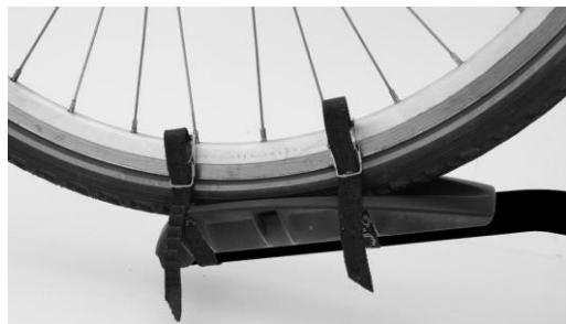
Secure the wheels using the supplied short straps. One strap for the fixation of the rear wheel and two straps for the front wheel (see picture).
